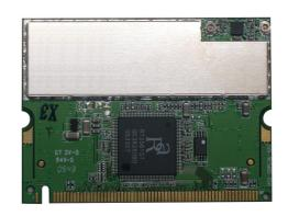
The **WCM6002** is a very small card that can fit into any notebook, handheld or desktop computer equipped with a Mini PCI (Type III B slot) interface for wireless network applications. It allows you to take full advantage of your notebook's mobility with access to real-time information and online services anytime and anywhere. It slides easily into the MINI PCI expansion slot to enable a wireless connection to your network.
